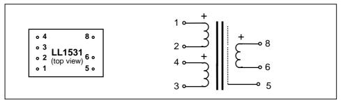
**Spacing between pins:** 3.81 mm (0.15") **Spacing between rows of pins:** 20.32 mm (0.8")
