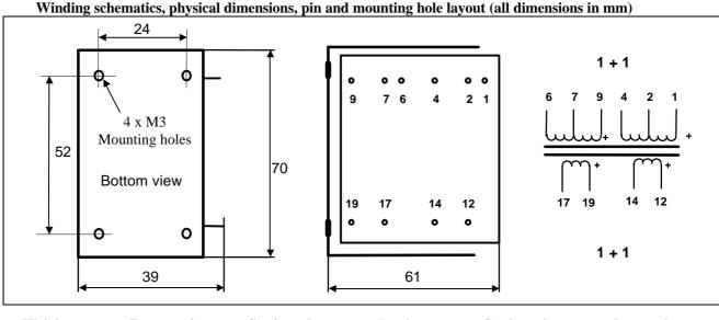
WeightTurns ratioStatic resistance, each primary0.5 Kg1+1:1+1 $500 \Omega$
