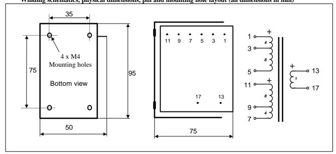
Weight: 1.35 kg Static resistance of each primary:  $102~\Omega$ **Static resistance of secondary:**  $0.4 \Omega$ 4 kV / 2 kV Isolation between windings / between windings and core: Max DC current through any primary winding: 160mA
