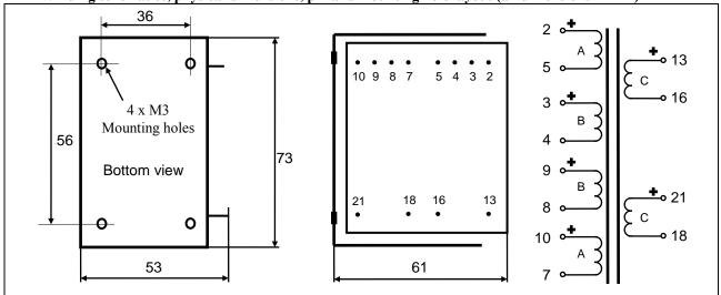
Max. current through any single section:  $$100\ mA$$  Isolation between primary and secondary windings / between windings and core:  $$4\ kV\ / 2\ kV$$
