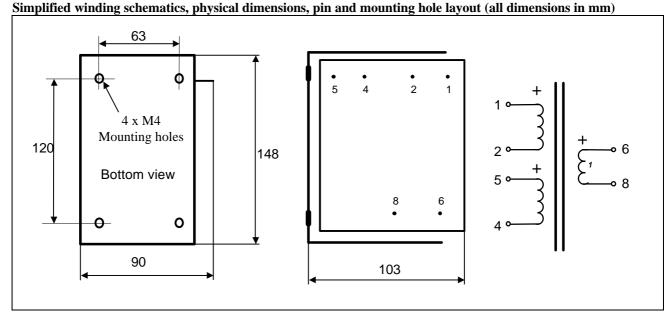
$\begin{tabular}{lll} Weight: & 4.6 kg \\ Static resistance of each primary: & 112 $\Omega$ \\ Static resistance of secondary: & 0.3 $\Omega$ \\ Isolation between windings / between windings and core: & 4 kV / 2 kV \\ Max DC current through any primary winding (10W heat dissip): & 210mA \\ \end{tabular}$
