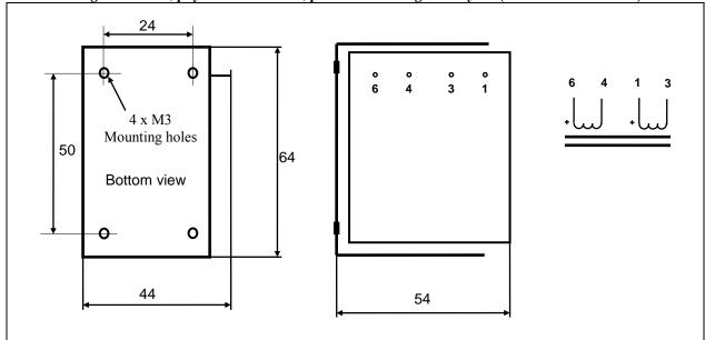
Weight:0.44 kgStatic resistance of each winding: $0.5 \Omega$ Isolation between windings / between windings and core:4 kV / 2 kV
