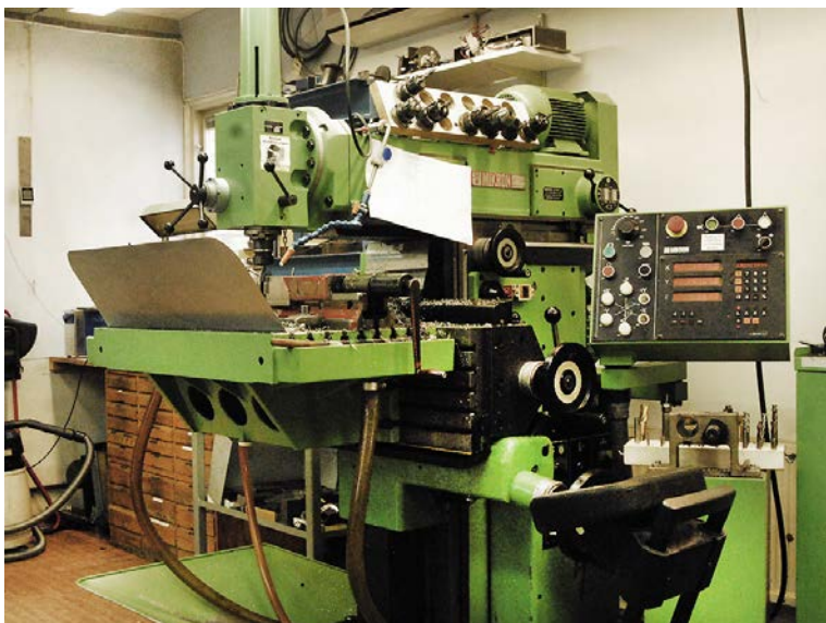
Figure 1: CNC milling machine in Lundahl’s machine tool fabrication shop where production equipment is designed and manufactured.
